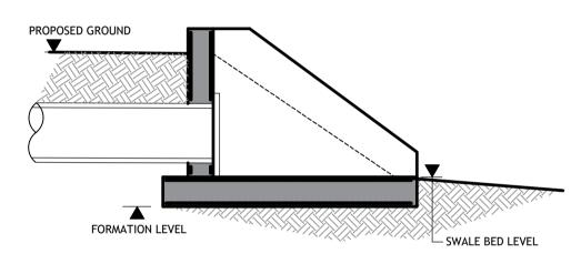
SWALE HEADWALL - SECTION SCALE 1:50
